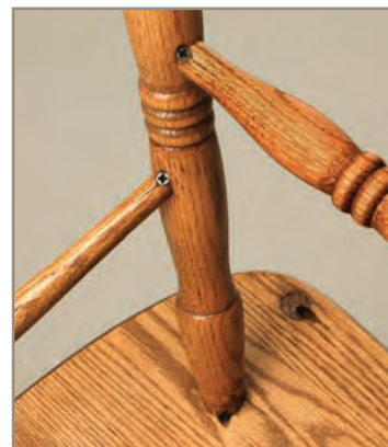
Joined using both screws and glue
