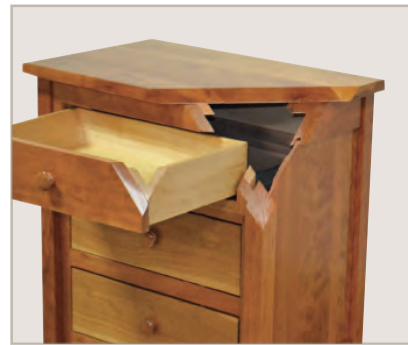
Fusion Designs uses floating panel construction . Rubber space balls are inserted into the frame so the wood panels can expand and contract without causing damage. Soft-close undermount drawer glides assure quiet operation of solid wood drawers.
