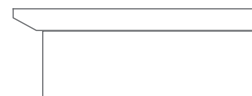
Top with Reverse Bevel SST-RB Adds 3/4" to overall height. Adds 2" to overall width. Adds 1" to overall depth.
