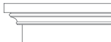
Top with Trim SMT-CH Adds \frac{3}{4} " to overall height. Adds 2" to overall width. Adds 1" to overall depth.
