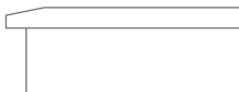
Top with Large Bevel SMT-LB Adds \frac{3}{4} " to overall height. Adds 1 \frac{1}{2} " to overall width. Adds \frac{3}{4} " to overall depth.
