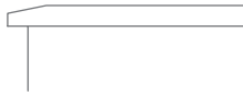
Top with Large Bevel SBT-LB Adds 1" to overall height. Adds 1½" to overall width.
