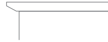
Top with Reverse Bevel SBT-RB Adds 1" to overall height. Adds 2" to overall width.
