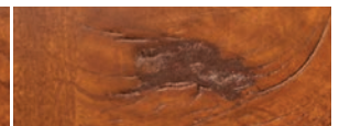
Character Cherry & QSWO Table Tops Filled Knots Standard Case Goods Tops Filled Knots Standard Chair Seats Filled Knots Standard
