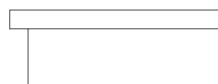
Top with \frac{3}{4} " Overhang SMT-TR Adds \frac{3}{4} " to overall height. Adds 1\frac{1}{2} " to overall width. Adds \frac{3}{4} " to overall depth.
