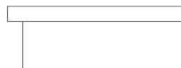
Top with 3/4" Overhang SST-TR Adds 3/4" to overall height. Adds 1½" to overall width. Adds 3/4" to overall depth.
