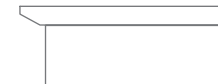
Top with Reverse Bevel SMT-RB Adds \frac{3}{4} " to overall height. Adds 2" to overall width. Adds 1" to overall depth.
