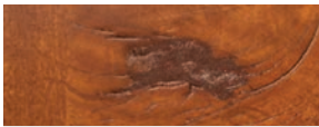
Character Cherry & QSWO Table Tops Filled Knots Standard Case Goods Tops Filled Knots Standard Chair Seats Filled Knots Standard
