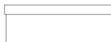
Top with \frac{1}{8} " Overhang SMT-MO Adds \frac{3}{4} " to overall height. Adds \frac{3}{4} " to overall width. Adds \frac{3}{8} " to overall depth.
